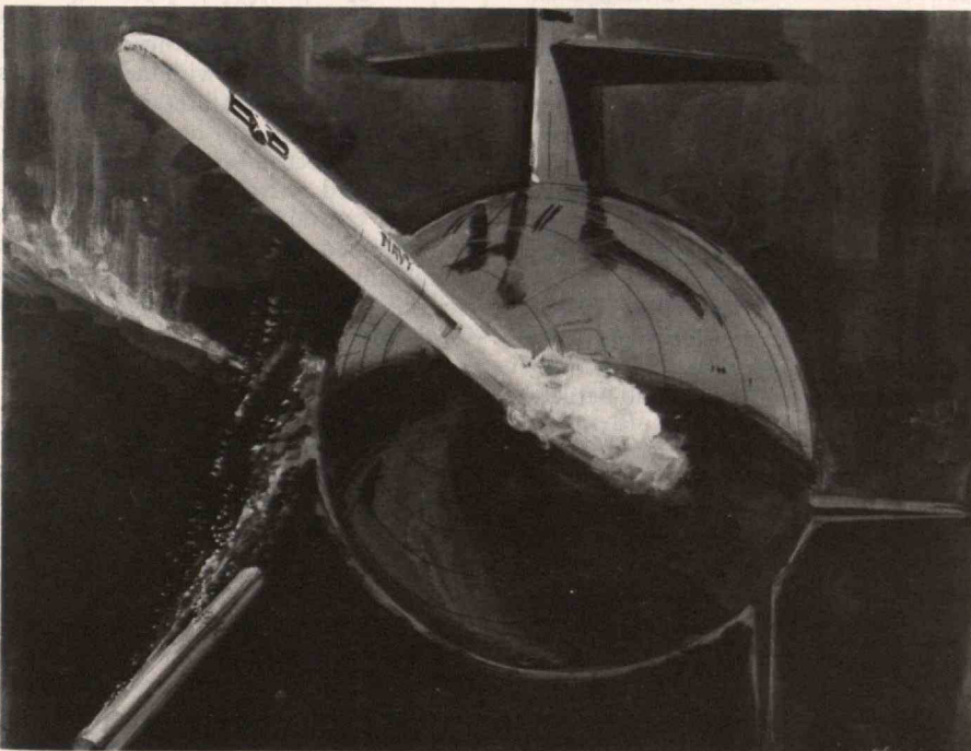
The Long-Range Cruise Missile can be fitted with a conventional warhead and used as a tactical weapon, or fitted with a nuclear warhead and used as a strategic weapon. Both could be launched, as shown in the artist's depiction, from the torpedo tube of a submarine. Since both would be encased in a protective stainless steel capsule (shown ejected to the left in the drawing), it would be "literally impossible to distinguish between the two versions without dismantling the weapon," according to Kosta Tspis, member of M.I.T.'s Center for International Studies. This, he feels creates a situation which would seriously hinder international arms limitation agreements. (Illustrations courtesy of General Dynamics)
