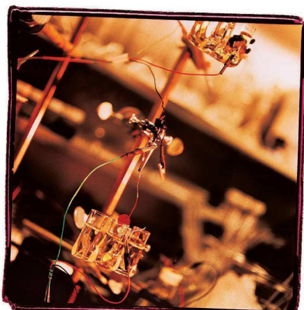
Manipulating polymers: Giaccai (top and left) fine-tunes the battery, which is enclosed in a glove box to protect it from moisture. The polymer 3,4,5 TFPT proves itself as an anode (right).
