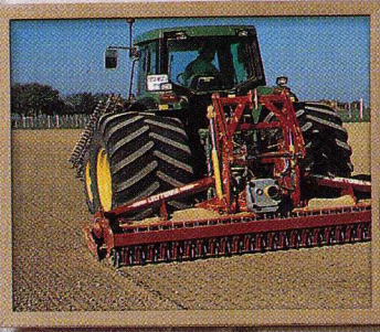
Michelin XM609, the widest available agricultural tractor tyre, provides real low ground pressure to prevent soil compaction
