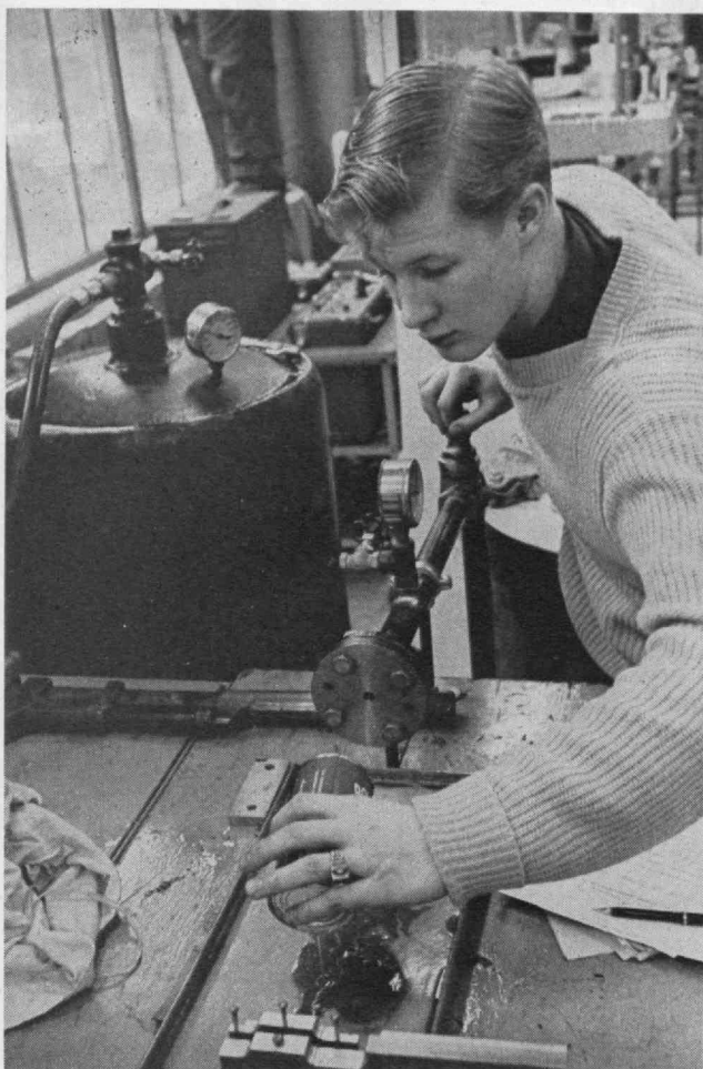
GEORGES S. DUVAL, 3d, '63 , at left, is comparing the power efficiencies of small-diameter rounded-entrance nozzles and sharp-edged orifices, with oil as a working fluid. Georges is shown preparing the instrumentation required to measure thrust associated with the nozzles and orifices.
